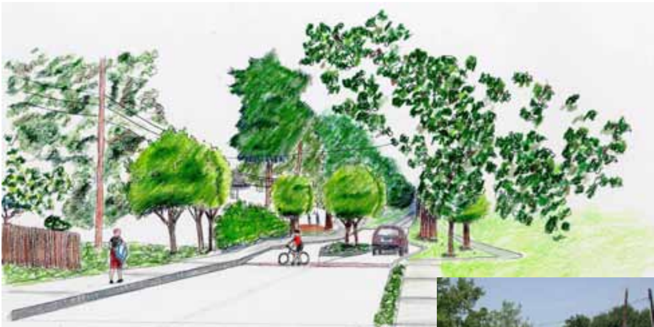
Figure 4-38: Existing (at right) and proposed splitter islands for Clay Street (above) to shorten the long sight lines as a method of self enforcing the posted speed limit
