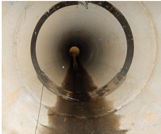
Figure 2-3. Bubbler flow module located at the midpoint of the Pond-R outfall pipe sampling stage data for the Pond-R station.
