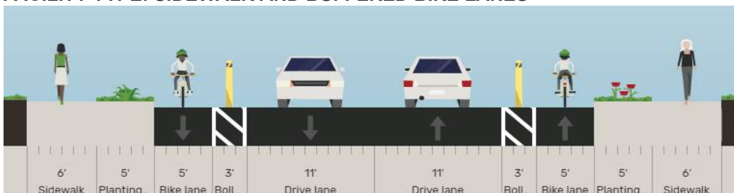
Figure 12: Buffered Bike Lanes (created using Streetmix.net)
