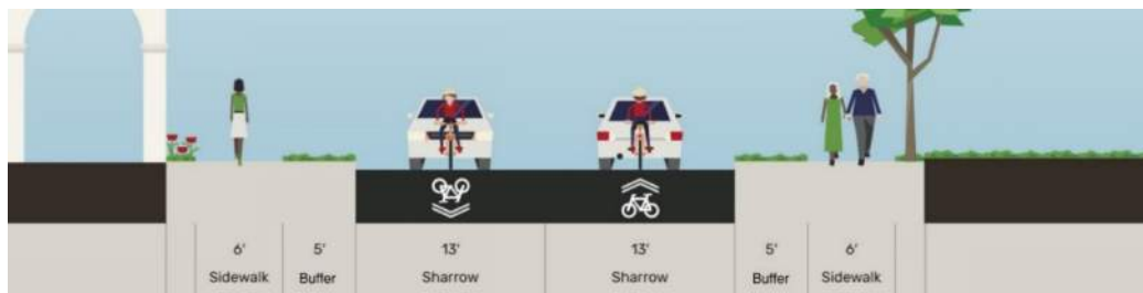
Figure 10: Shared-Lanes Typical Section (created using Streetmix.net)
