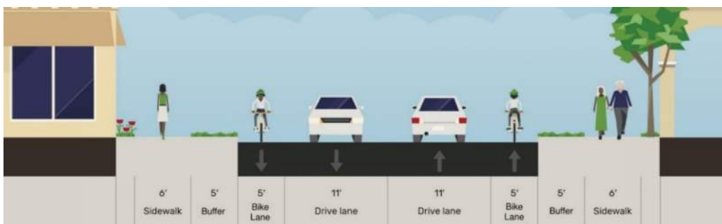
Figure 11: Bike Lanes Typical Section (created using Streetmix.net)
