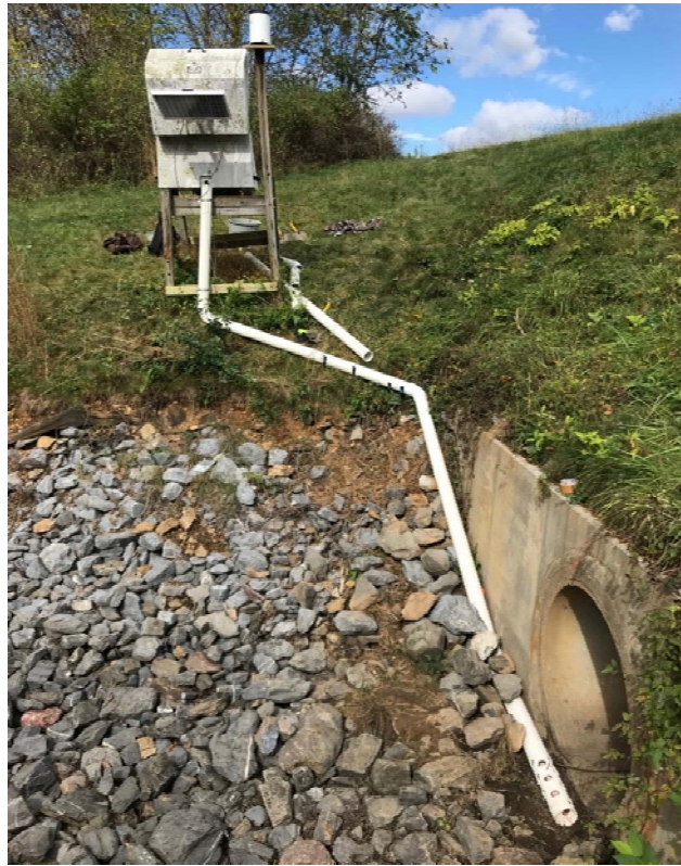
Figure 2-2a. Villages of Urbana “Pond-R” outfall water chemistry monitoring station and rain gauge. Photograph taken October 16, 2017.
