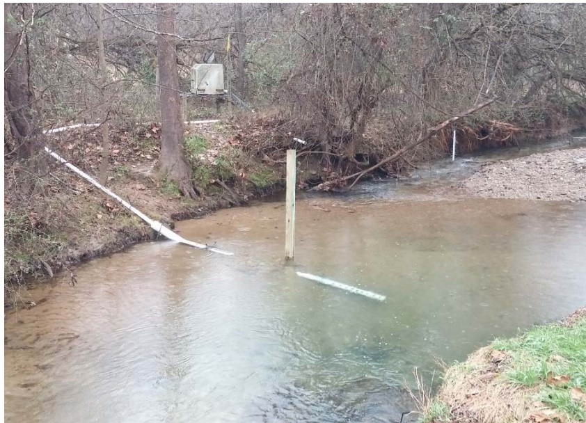
Figure 2-1. Ambient instream monitoring station at Peter Pan Run in the Lower Bush Creek watershed, Frederick County, MD. The instream station includes sample intake tubing located near a stilling well at the center of the stream, a staff gauge and flow meter sensor against the left bank, and a “storm box” located in a clearing near the bank. Photograph taken November 24, 2018.
