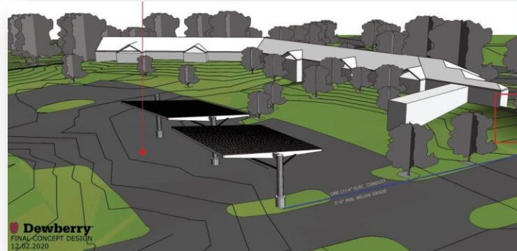
The Bourne Building houses offices for the Public Works and Parks and Recreation Divisions. Initial plans call for two sets of panels to be erected in the parking lot on the north side of the building. Each structure will house 84 solar panels, for a total of 168 panels. Design work begins this month. The project will go out for bids later this year, with construction expected to begin next spring.
