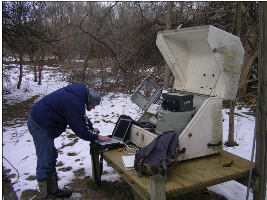
Figure 2-1a. The “storm box” at the ambient instream monitoring station at Peter Pan Run in the Lower Bush Creek watershed, Frederick County, MD. The storm box contains an ISCO sampler, streamflow meter, battery, and a data recording unit. Photograph taken in January 2010.
