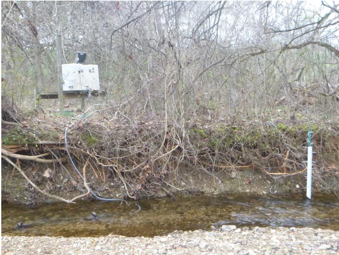
Figure 2-1b. Ambient instream monitoring station at Peter Pan Run in the Lower Bush Creek watershed, Frederick County, MD. The instream station includes sample intake tubing located in the center of the stream, a staff gauge and flow meter sensor against the left bank, and a “storm box” located in a clearing near the bank. Photograph taken in December 2015.
