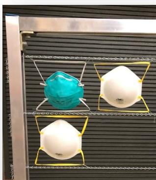
*Photos (from top): The prototype ultraviolet system created by Frederick County staff. An interior view of the decontamination unit. N95 masks hang on racks that are placed inside the unit.*
