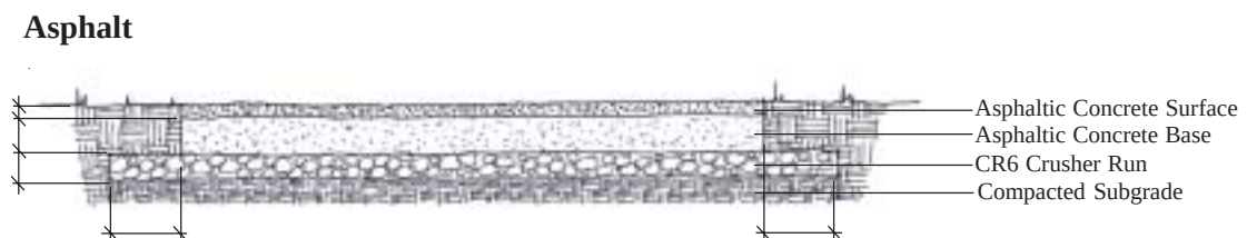
Figure 7 Typical Asphalt Paving Section (Exact dimensions to be determined)
