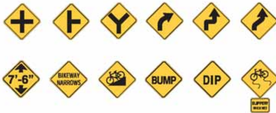
Figure 22 Examples of Warning Signs
