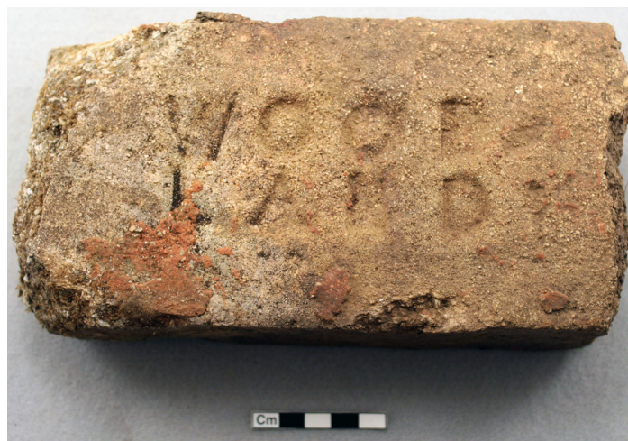
Firebrick discarded during routine blast furnace relining at Catocin Iron Furnace, Frederick County. This brick was manufactured by Woodland Fire Brick Co, Clearfield Co., Pennsylvania. Image courtesy of Elizabeth A. Comer.
